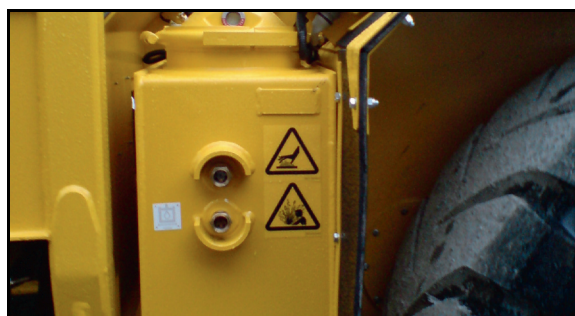
Hydraulic oil tank (sight glass)
